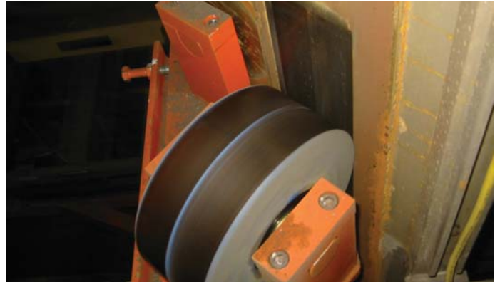
Floor-to-floor elevator guide wheel of NYTEC-HS
