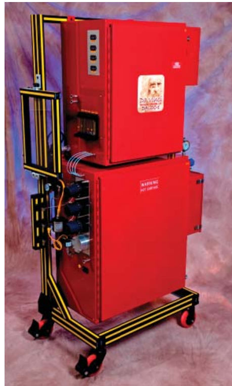
CASTERSHOX CASTERS WERE USED ON OIL CONSUMPTION CARTS TO ELIMINATED THE CRACKING OF THE PREVIOUS SWIVEL SECTIONS AFTER A FEW MONTHS OF USE.
